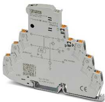
3-conductor with common reference potential, 3/6 connection grounded via gas-filled surge arrester, one-piece
